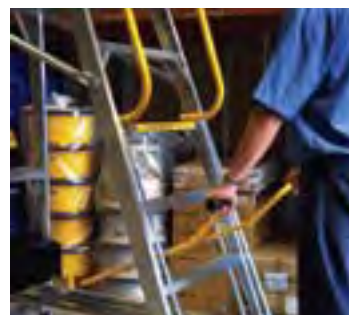
Ergonomically designed lift and steer control handle.
