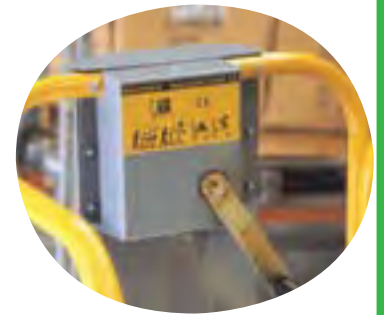
User friendly hand winch operation allows operator to raise and lower loads of up to 60kg
